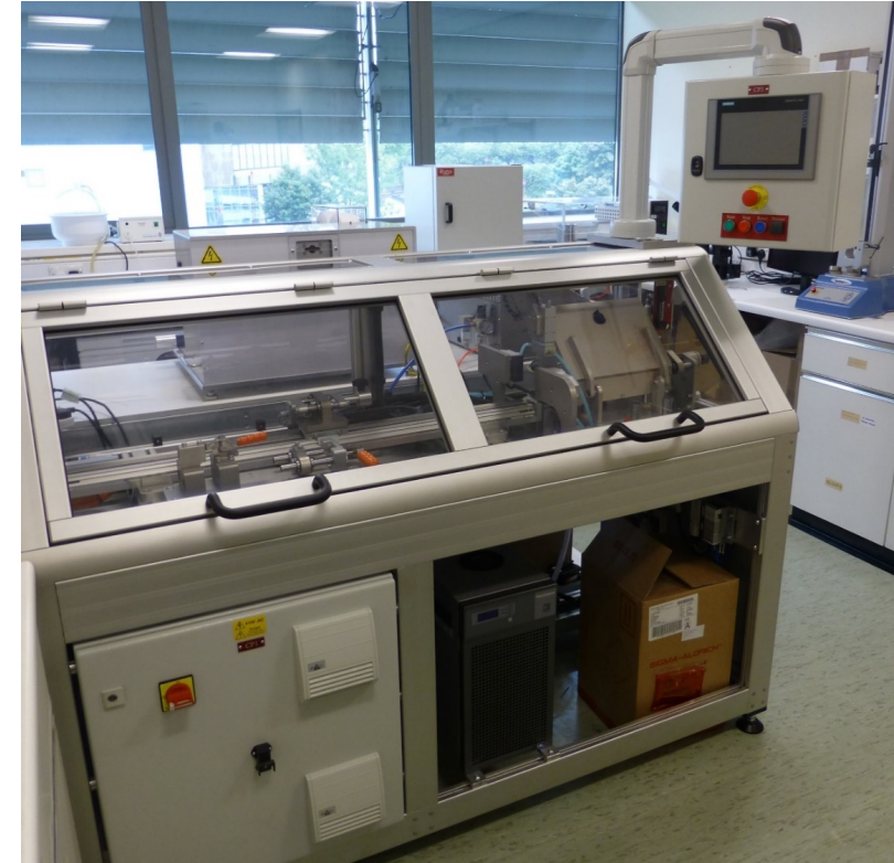
Arterius die drawing system produced in 2016 used for development and production
