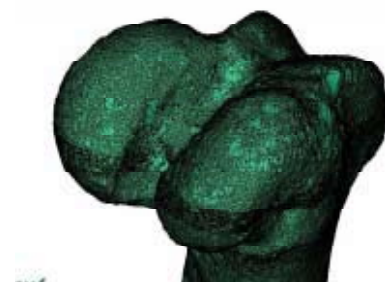
Finite element model, constructed from laser scanning, of a sheep's knee, for optimisation of articulating surface implant geometry.
