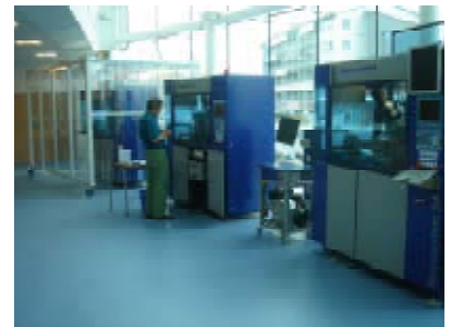
Smart Point production on one of the Battenfeld high precision micromoulding machines at Bradford.
