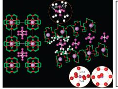
The first sodium conducting crystalline polymer electrolyte, PEO<sub>8</sub>: NaAsF<sub>6</sub>, which has a conductivity 1.5 orders of magnitude higher than PEO<sub>6</sub>:LiAsF<sub>6</sub> at 25<sup>o</sup>C The structure of PEO<sub>8</sub>: NaAsF<sub>6</sub>, from the single-crystal data collected at 25<sup>o</sup>C, Left: view of
