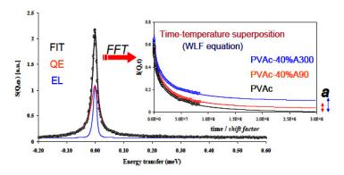
QENS spectra of PVAc containing 40 wt% A300 as measured on IRIS at 478K and Q = 1.45 Å<sup>-1</sup>, the fit to the experimental data including a quasielastic and an elastic contributions. Inset: overlapped Intermediate scattering function I(Q,t) data of bulk and nanoparticle filled PVAc as well as their fits at 1.58 Å<sup>-1</sup> (reference temperature: 478 K).
