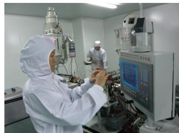
*Industrial extrusion line of multi-layer medical tube,
