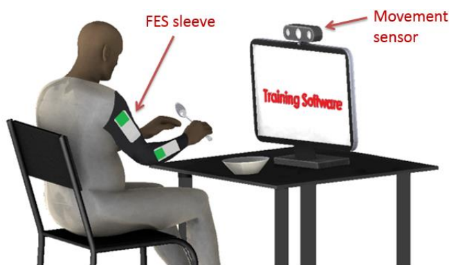
Figure 3. FES training system for stroke upper limb rehabilitation
