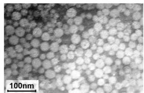
TEM micrograph of PS latex obtained through ultrasonically induced microemulsion polymerization of St (Chuhong Zhang, Qi Wang, Hesheng Xia, Guihua Qiu, European Polymer Journal 38, 1769, 2002)
