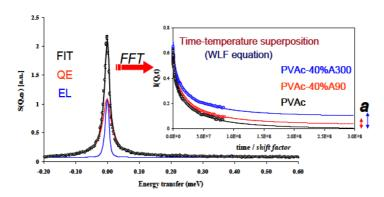
QENS spectra of PVAc containing 40 wt% A300 as measured on IRIS at 478K and Q = 1.45 Å<sup>-1</sup>, the fit to the experimental data including a quasielastic and an elastic contributions. Inset: overlapped Intermediate scattering function I(Q,t) data of bulk and nanoparticle filled PVAc as well as their fits at 1.58 Å<sup>-1</sup> (reference temperature: 478 K).
