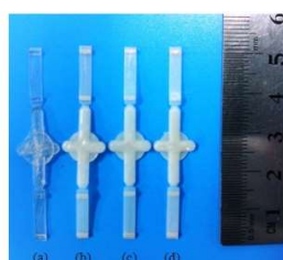
Micro-injection samples of PVA/n-HA composites. (a) PVA, (b) 10%HA, (c) 20%HA, (d) 30%HA.
