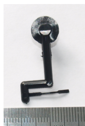
Electrical conductive and flexible PU/CNTs micro-molded parts
