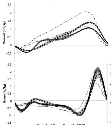
External moment and mechanical power at distal end of shank (mean  $\pm$  SD across 10 trials) when using hydraulic ankle articulating device (dark shading) versus fixed ankle (light shading).
