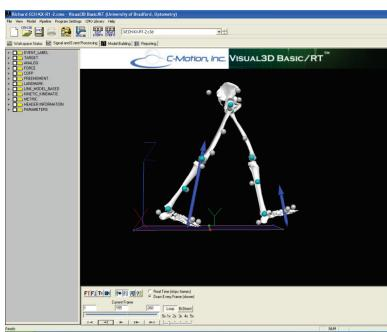
Biomechanical modelling of data collected via 3D motion capture
