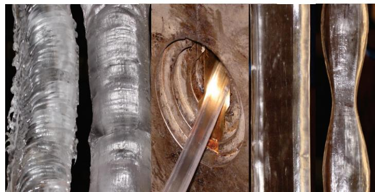
Observe how an increase in roller speeds stabilise extrudate. For principles see: Benkreira et al, *International Polymer Processing*, 2004, 19(2), 111-117
